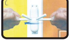
E. Using the steel bar supplied to adjust the tension turn the centre boss away from the door or gate. Locate the hole nearest the door or gate and screw in the arm. Repeat this operation one hole at a time to increase the tension.
